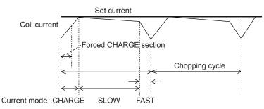
Charge mode continues until  $I_{COIL} \ge I_{REF}$ . After that the IC switches to SLOW DECAY mode and then switches to FAST DECAY mode for the last about 1 $\mu$ s.
