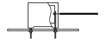
Temperature monitored inside the capacitor.
