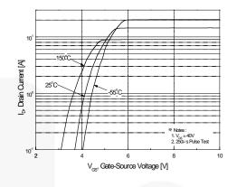
Figure 2. Transfer Characteristics
