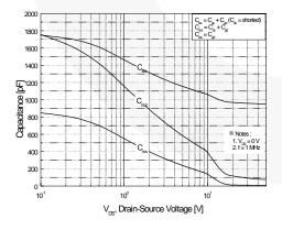
Figure 5. Capacitance Characteristics
