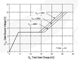
Figure 6. Gate Charge Characteristics
