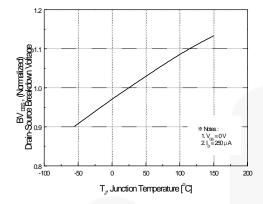
Figure 7. Breakdown Voltage Variation vs Temperature
