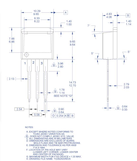
Figure 17. TO262 (I<sup>2</sup>PAK), Molded, 3-Lead, Jedec Variation AA
