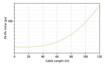
Figure 2-3: Jitter vs. Cable Length (2970Mb/s)
