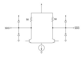
Figure 3-3: Output Circuit
