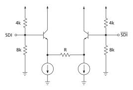
Figure 3-1: Input Equivalent Circuit
