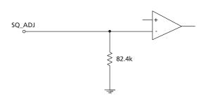
Figure 3-2: SQ\_ADJ Equivalent Circuit
