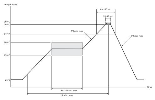
Figure 6-1: Maximum Pb-free Solder Reflow Profile
