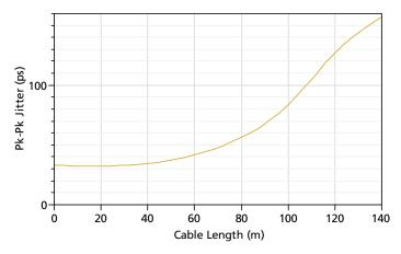
Figure 2-2: Jitter vs. Cable Length (1485Mb/s)
