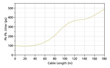
Figure 2-1: Jitter vs. Cable Length (270Mb/s)
