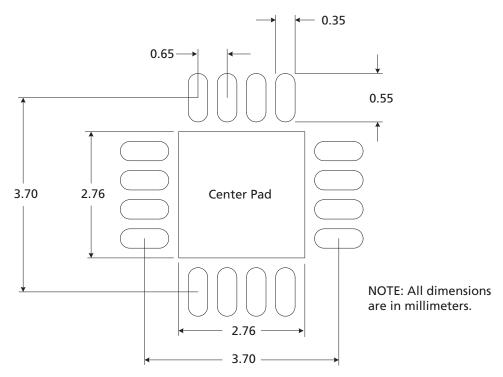
The Center Pad should be connected to the most negative power supply plane for analog circuitry in the device (VEE\_A) by a minimum of 5 vias.
