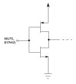
Figure 3-4: MUTE and BYPASS Circuits
