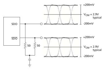
Figure 4-1: Typical Output Voltage Levels
