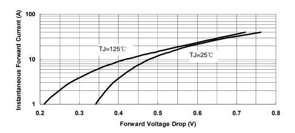
Fig.3-Typical Instantaneous Forward Voltage Characteristics
