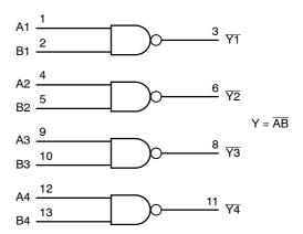
Figure 2. Logic Diagram
