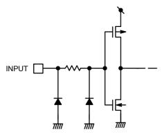
Figure 7. Input Equivalent Circuit
