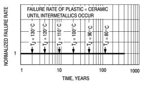
Figure 4. Failure Rate vs. Time Junction Temperature
