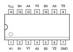
Figure 1. Pin Assignment (Top View)
