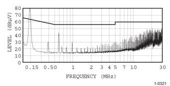
Figure 9. HW050FG Conducted Noise with Filter Compared to Class B Limits
