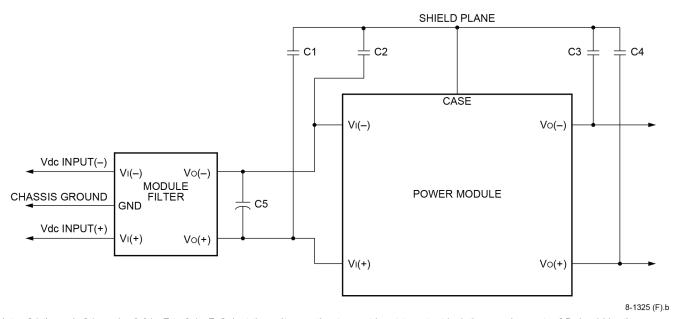
Note: C1 through C4 can be 0.01 μF to 0.1 μF. Select the voltage rating to meet input-to-output isolation requirements. C5 should be the recommended value indicated in the power module data sheet.
