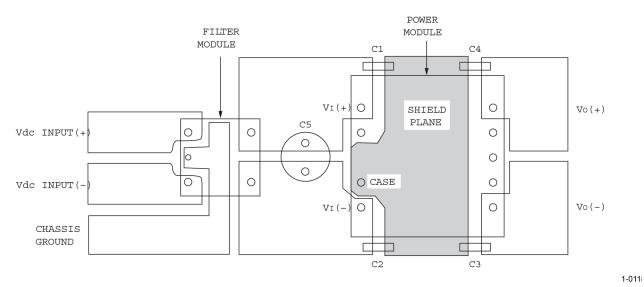
Note: Vdc input(+) and Vdc input(-) planes should overlay each other, as should the VI(+) and VI(-) planes, as should the VO(+) and VO(-) planes. Avoid routing signals or planes under the power module or the filter module. Ensure all connections are low impedance.
