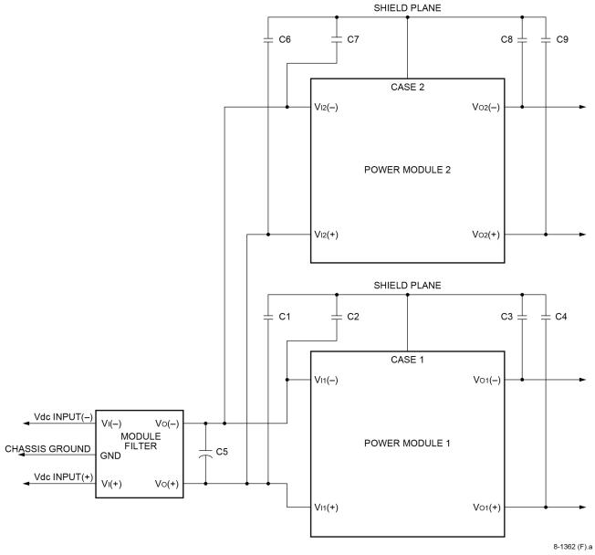
Note: C1 through C4 and C6 through C9 can be 0.01  $\mu$ F to 0.1  $\mu$ F. Select the voltage rating to meet input-to-output isolation requirements. C5 should be the recommended value indicated in the power module data sheet.
