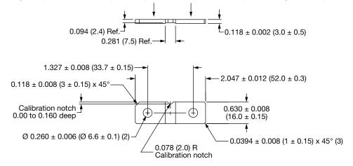
Plating on top / bottom is Sn 2.5 µm to 8.0 µm over Ni 0.5 µm to 4.0 µm, punched edges are not plated
