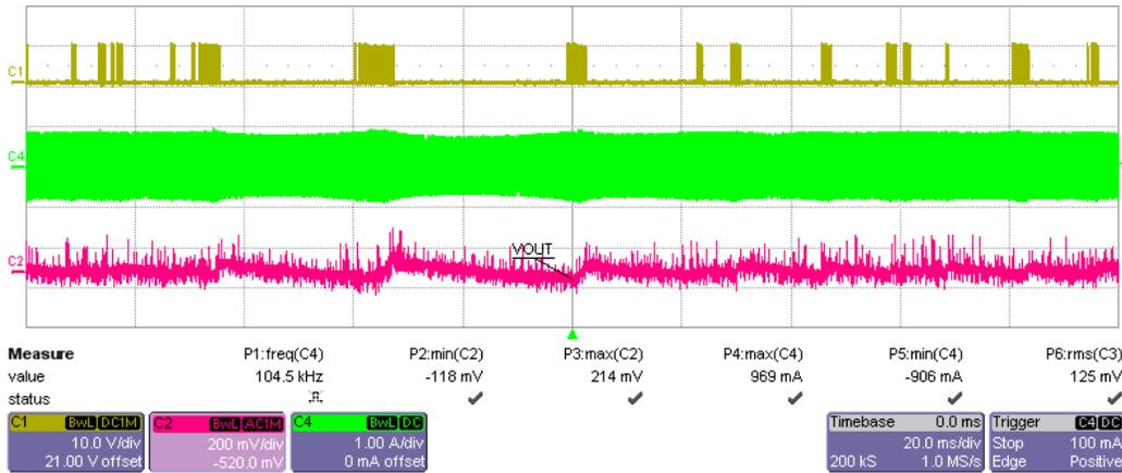
IR11682 in burst mode at 390Vdc, no load.
