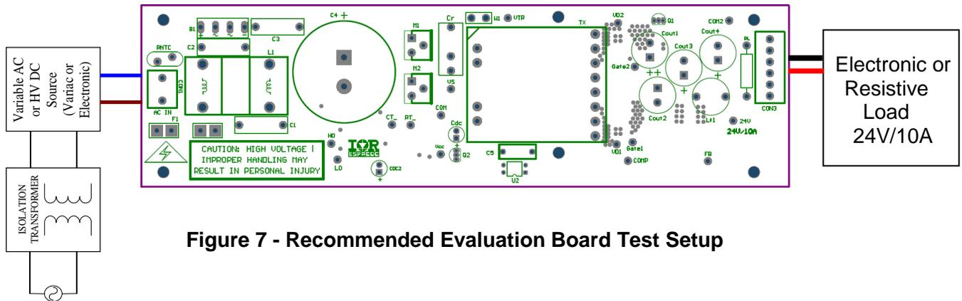
Figure 7 - Recommended Evaluation Board Test Setup
