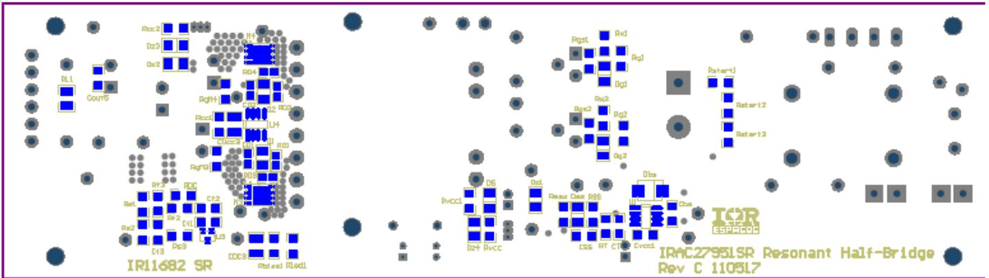
Figure 4 – Evaluation Board Bottom Side Component Placement
