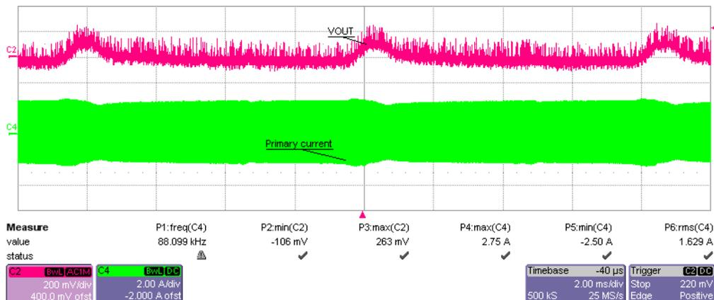
The ripple is mainly due to the low frequency (2xfAC) ripple on primary bus voltage. It will be much smaller if use a PFC pre-regulator in the front stage.
