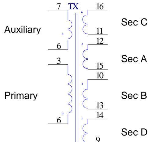
*Note: pin9 is shorted to pin10 on PCB, pin12 is shorted to pin13 on PCB and pin15 is shorted to pin16 on PCB.*
