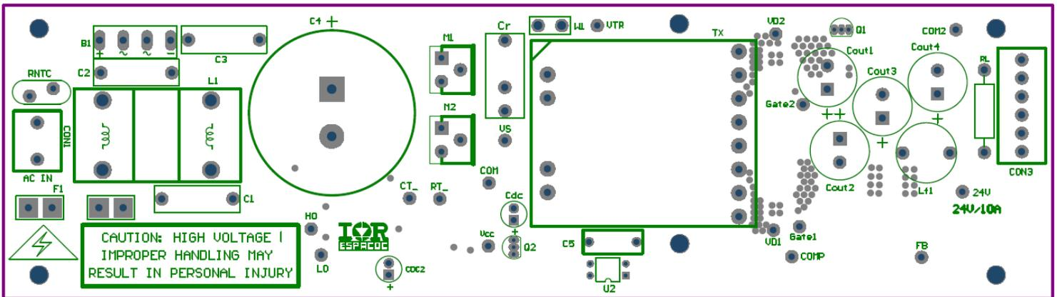
Figure 3 – Evaluation Board Top Side Component Placement
