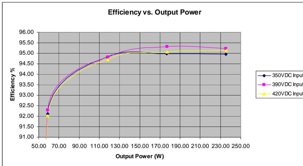
Figure 9 - Efficiency plot
