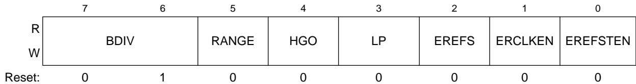
Figure 11-4. ICS Control Register 2 (ICSC2)
