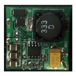
Figure 1. NCV8852GEVB Board Picture
