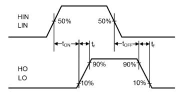
Figure 3. Switching Time Waveform Definitions
