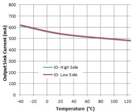
Figure 19. Output Sink Current vs. Temperature
