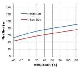
Figure 9. Rise Time vs. Temperature
