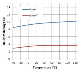
Figure 15. Delay Matching vs. Temperature
