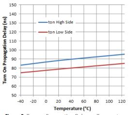
Figure 5. Turn-on Propagation Delay vs. Temperature
