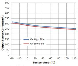
Figure 17. Output Source Current vs. Temperature
