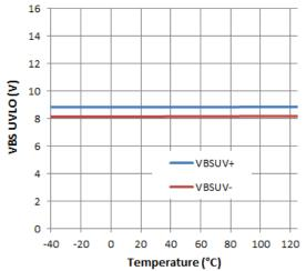
Figure 25. VBS UVLO vs. Temperature
