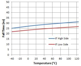
Figure 11. Fall Time vs. Temperature
