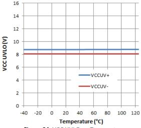
Figure 24. VCC UVLO vs. Temperature
