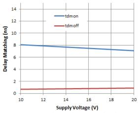
Figure 14. Delay Matching vs. Supply Voltage
