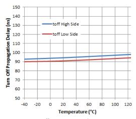
Figure 7. Turn-off Propagation Delay vs. Temperature
