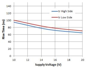
Figure 8. Rise Time vs. Supply Voltage
