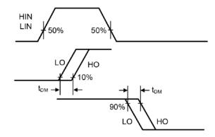
Figure 1. Input / Output Timing Diagram
