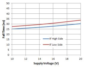
Figure 10. Fall Time vs. Supply Voltage
